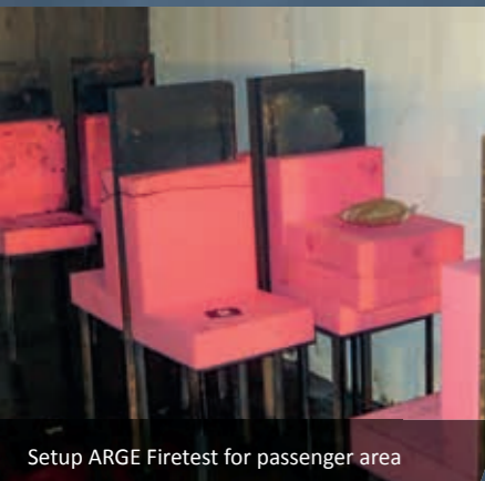
Fire test according UNI11565 including luggage rack
